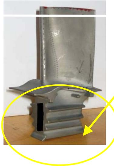
The HP turbine blade root mass, size, and tangential velocity make it a very significant fragment.
